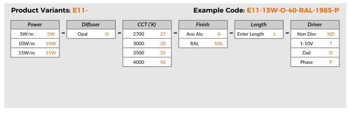
NB Compatibility of the phase dimmer and driver must be checked prior to order
